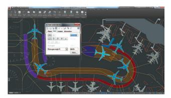
>> Perform jet blast studies to ensure ground personnel and equipment are safe from high wind speeds aft of moving airplanes
