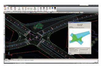
>> With grading applied, the intersection design's high and low points can be analyzed in a three dimensional way.
