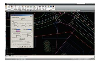
>> Easily generate vehicle movements for the intersection and adjust the geometric design accordingly.
