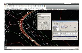
>> Place vehicle simulations on a specific level/layer and use different colors, line styles, and drawn options for swept path envelopes and vehicle components.
